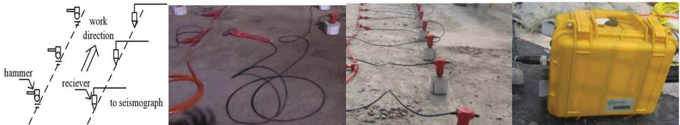
FIG. 11 Equipment for acquisition work in field (a) before grouting and (b) after grouting.
